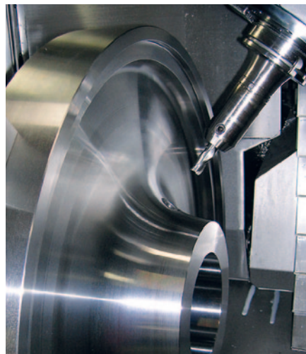
Turning and milling a wheel-set disk
