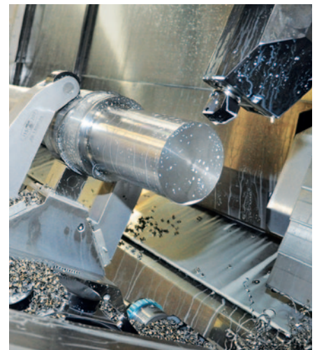
Turning a wheel-set axle
